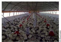
Fig.7.10: Opened building with natural ventilation.
