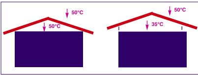
Fig.7.6: Roof edge overhanging to protect the walls. A wall in the shade receives 30% less radiant heat than a wall in the sun.
